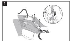
Remove the radiator scoops. Disconnect the fuel pump cover cable and the fuel connector as indicated in the diagram. Replace the original breather pipe with the one in equipment (I).
