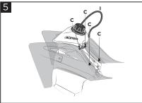
Assemble the radiator scoops with the screws (C). Connect the tube (I) to the cap
