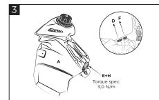
On the fuel tank Acerbis (A), reconnect the fuel pump (E) using the screws (H) with the original hardware.
