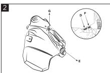
Remove the tank screw (G), then empty any remaining fuel from the tank. Remove the (D/E/F) fasteners and remove the fuel pump.
