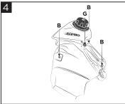
Place the Acerbis fuel tank (A) on the bike. Insert the tank and seat screws (G/B) as indicated in the diagram. Reconnect the fuel pump power cable and the fuel connector.
